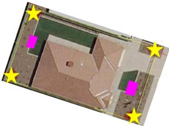
IP connections ★ are usually located near the property septic tank (shown in pink) and close to the boundary
